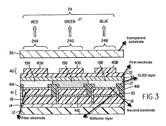
As to claim 2, Cok discloses the display wherein the organic electroluminescent display panel further comprises: a transparent substrate (Figure 3, element 36); a first transparent electrode (Figure 3, element 30) over the transparent substrate; a light-emitting layer (Figure 3, element 19) over the first transparent electrode; and a second transparent electrode (Figure 3, element 18) over the light emitting layer.
